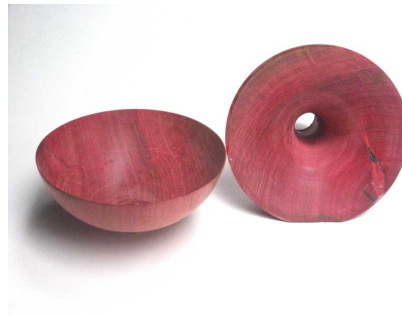
Note black defect in flange – this will disappear in piercing
