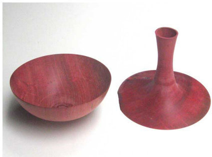
Top and bottom sections prior to gluing together
