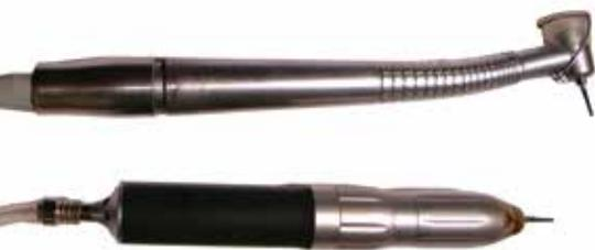
Air-powered tools: dental drill (top) and NSK tool.
