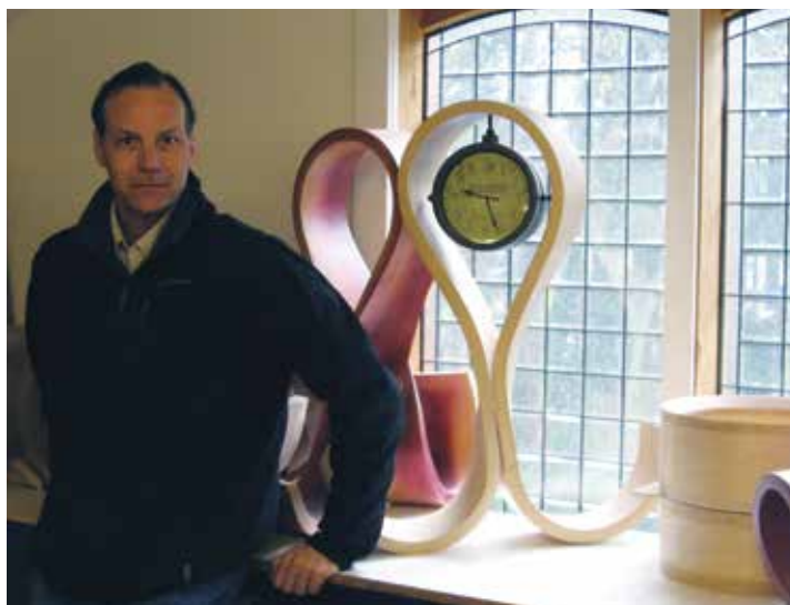
Chris Mroz, of Pure Timber, LLC, a supplier of compressed wood products, with a clock frame of 1.25" (32mm) compressed oak bent with mechanical leverage to a 6" (15cm) radius. Also pictured are snare drums made of bent compressed wood.
